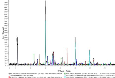
Figure 4. XRD analysis of pellets 3 after heat treatment.
