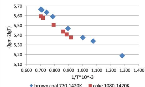
Figure 7. The dependence of  $\lg m - 2\lg T = f(1/T)$  of pellets 2 and 3 up to temperature 1420 K.
