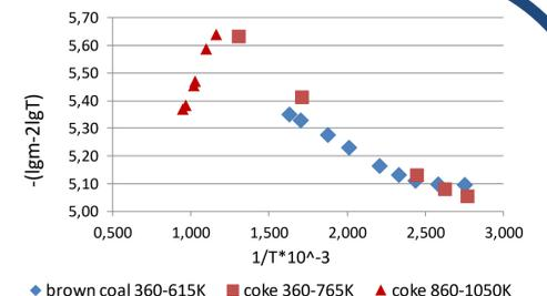
Figure 6. The dependence of  $\lg m - 2\lg T = f(1/T)$  of pellets 2 and 3 up to temperature 1050 K.
