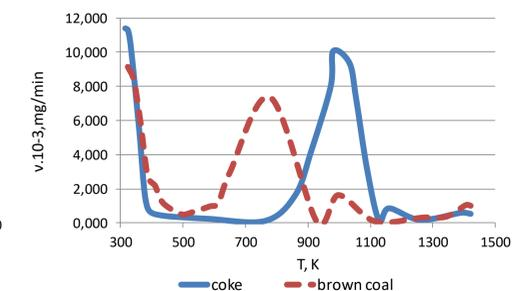
Figure 8. Rate of the processes depending on the temperature of the pellets containing reducer agent.
