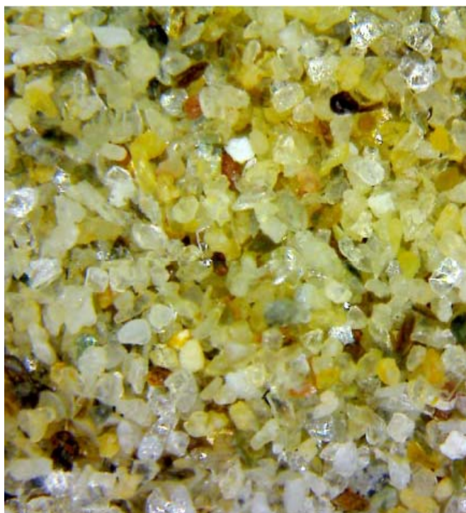
Figure 3. Microscopic appearance of fraction 0.250 / 0.125 mm, binocular magnification 40X
